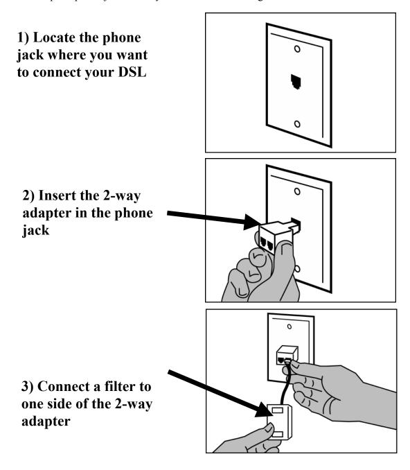
4) If you have a phone, fax machine, analog modem or other phone device at this location, connect it to the filter
